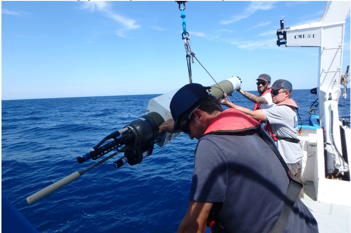
Deployment of an Argo profiling float equipped with a pH sensor at the DYFAMED site.
